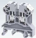
CTT2.5U Type 'K' / 'J' / 'T' / 'E' 0.2 - 2.5 mm 2 10 A, 1000 V, 0.4 Nm
