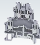
ODLG2.5 / ODLG2.5A 59.8 x 62 x 5 mm 0.2 - 2.5 mm 2 24 A, 800 V, 0.5 Nm
