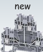
CYDL4(I.S) 65 x 70.5 x 6 mm 0.2 - 4.0 mm 2 32 A, 1000 V, 0.5 Nm
