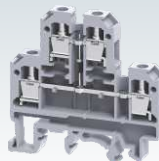
CDL4U(E) (Diode) 54 x 55.5 x 6 mm 0.2 - 4.0 mm 2 32 A, 500 V, 0.5 Nm
