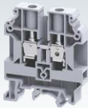
CHV10U 62 x 52 x 10 mm 0.2 - 10.0 mm 2 57 A, 1000 V, 1.2 Nm
